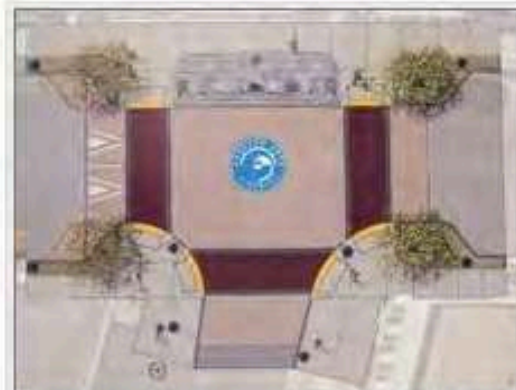
The new intersection will be raised to improve visibility. It will include landscaped bump outs and three, faux-
