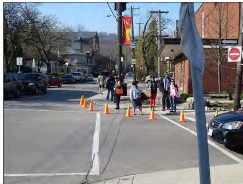
Pylon bumpouts at Herkimer and Locke (RTH file photo)
